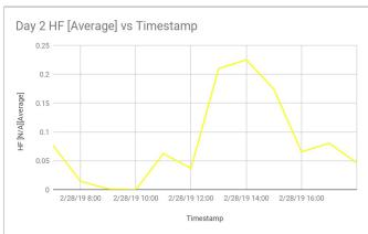
The HF emissions were compliant with the licence limits with a peak on Day 2 corresponding to a peak in flow rate of PFAS liquid injection between 12:45 and 15:45.
