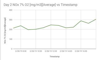
The NOx emissions were compliant with the licence limits during Day 1 and 2 of the trial.
