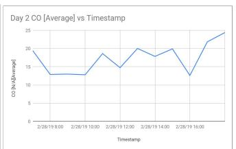
The measured emissions of carbon monoxide during the liquid trial burns were compliant with the EPA licence. No notable peaks could be noticed corresponding to the influence of PFAS injected.
