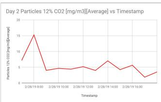
The emissions of particles exceeded the licence limit around 1pm of Day 1 of the liquid trial burn. They were compliant on Day 2 throughout. The Day 1 emissions do not correspond to any notable event relating to the trial, other than a load of confidential waste loaded prior. Moreover, the injection flow rate was much higher on Day 2 so the non-compliance could not easily be attributed to the injection of PFAS liquid.
