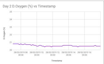
The level of oxygen in the combustion gases were compliant with the 10% minimum limit.
