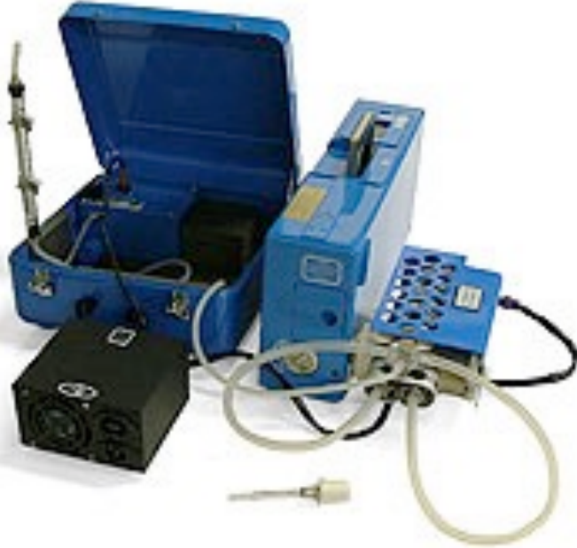
Ohio Lumex RA915+ Portable Mercury Vapor Analyser, which can also be adapted to sample soil and water.
