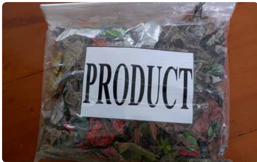
Figure 40. RDF fluffs samples from Jeruklegi Landfill, Cilacap Regency analysed in the lab. Photo: Nexus3
