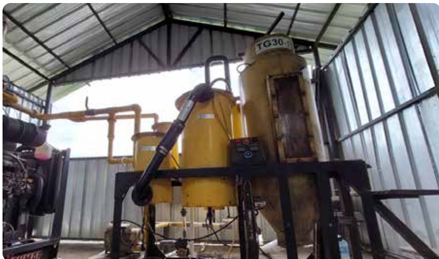
Figure 25. Gasification plant to generate electricity for machineries at TOSS facility in Klungkung. Photo: Nexus3
