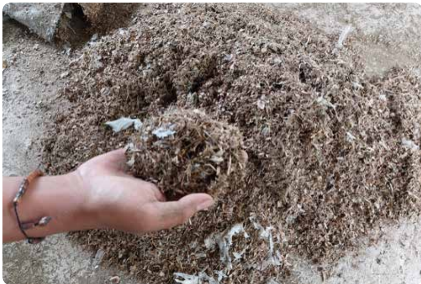
Figure 33. RDF in a form of shredded waste is now the end products of RDF Kebon Kongok. Photo: Nexus3
