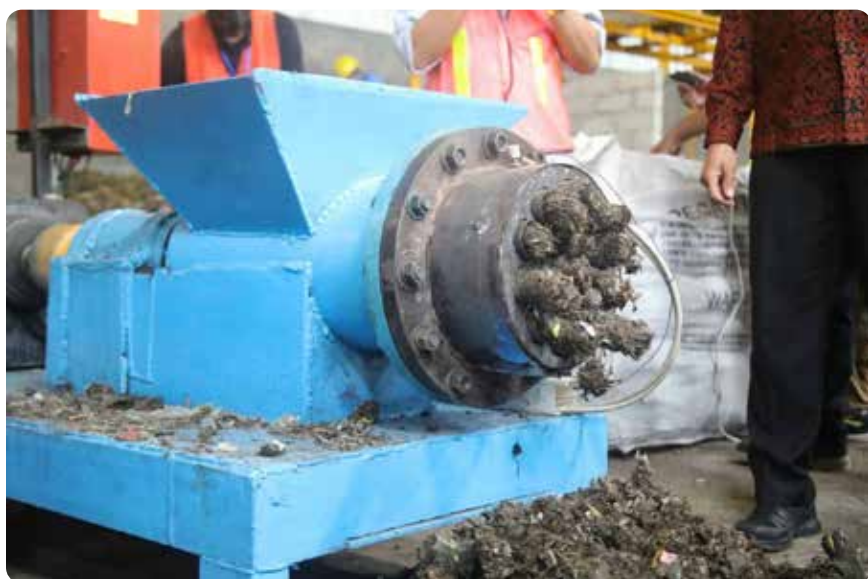
Figure 38. RDF pellets from mixed residues produced at TPST Samtaku Jimbaran will be sold to SMEs laundry and tofu factories. Photo: Kemenkomarves
