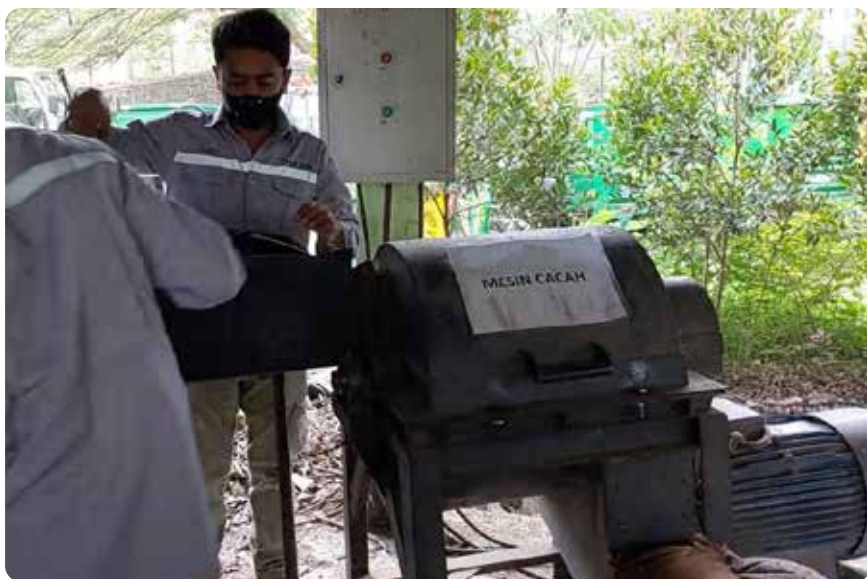
Figure 32. Dried wastes will be shredded into unspecified sizes. Photo: Nexus3
