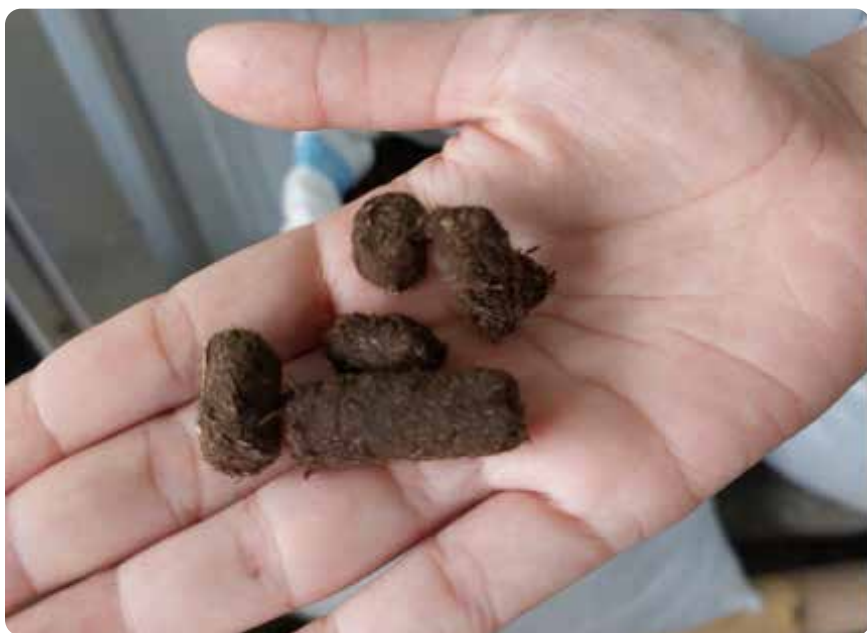
Figure 26. Example of RDF pellets produced by TOSS Centre in Klungkung. Photo: Nexus3
