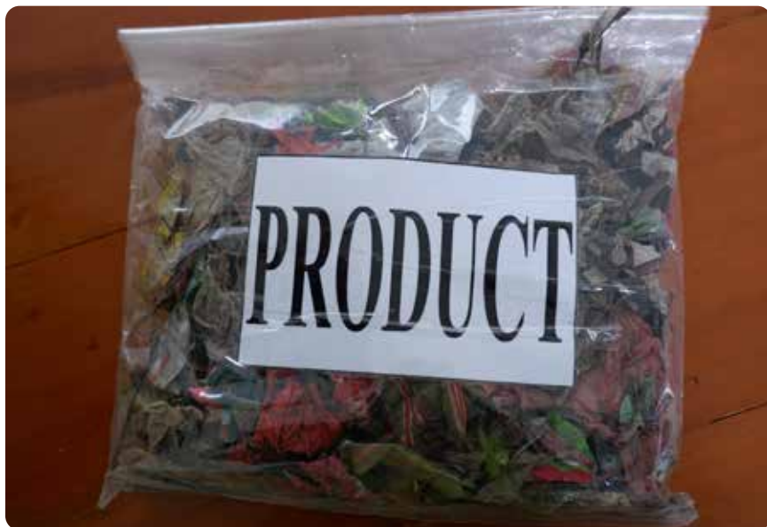
Figure 20. About 40-60 tons of RDF fluff products produced daily to be used at the cement kilns. Photo: WALHI
