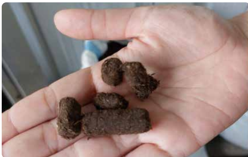
Figure 39. RDF pellet samples from TOSS Gema Santi, Klungkung Regency analysed in the lab. Photo: Nexus3
