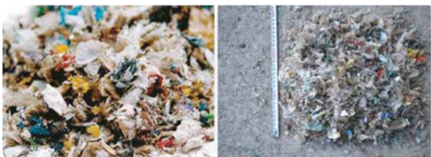
Figure 13. Example of RDF fluff for co-firing in cement kiln. Photo: Holcim, 2015
