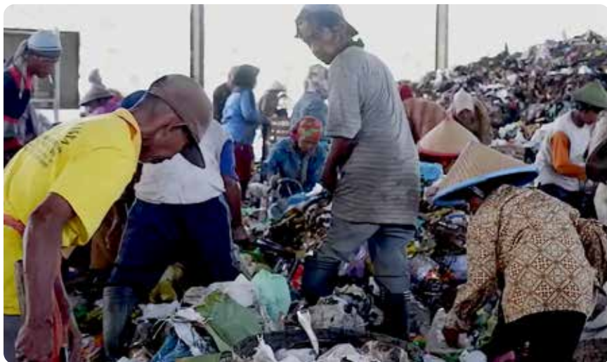
Figure 18. About 70-90 scavengers sorted 120 ton of waste per day and collected 3% of recyclables from the piles dropped at the RDF reception facility. The remaining wastes are the RDF feedstock. Photo: WALHI
