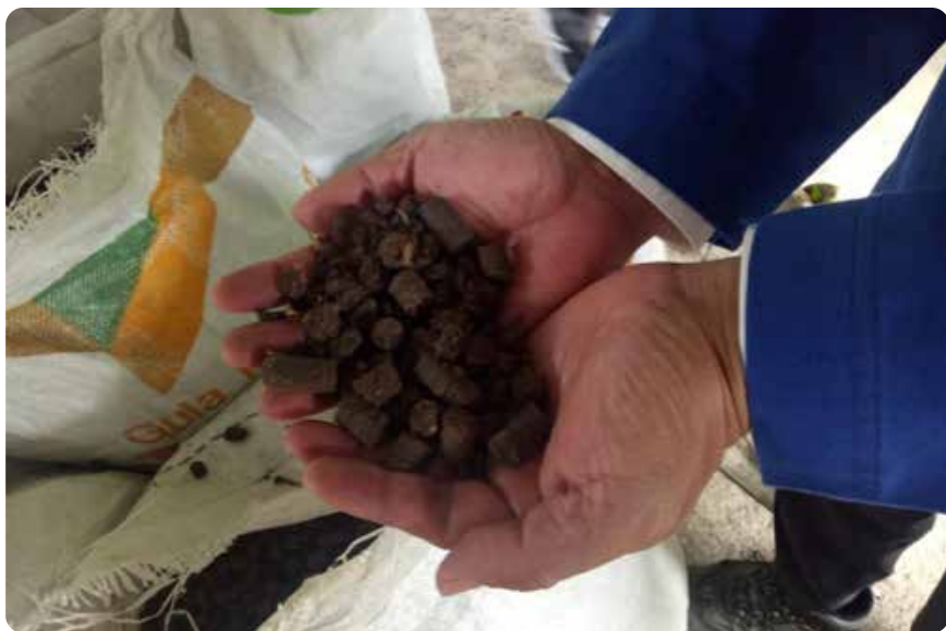
Figure 34. Initially this kind of RDF pellets will be used by PLTU Jeranjang. Photo: INA News
