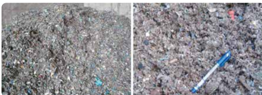
Figure 14. Example of RDF in form of Compost Like Output (CLO). Photo: Holcim, 2015
