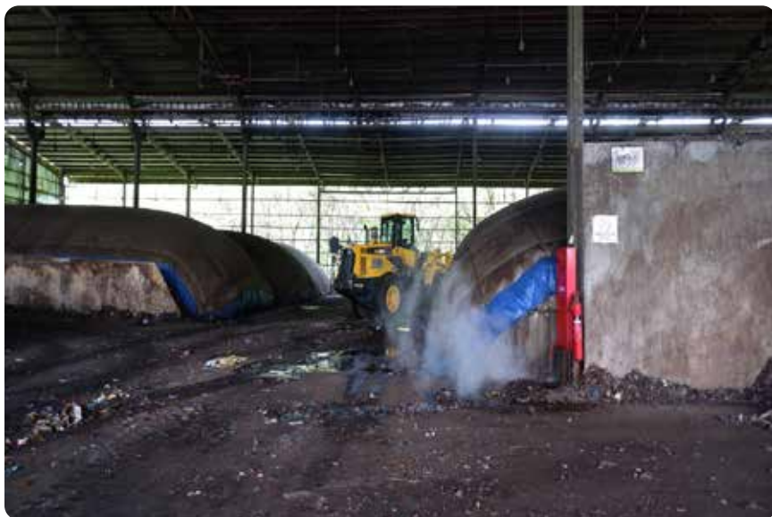
Figure 19. The RDF materials treated for 21 days at the Biodrying bays to reduce 35% of humidity in the RDF materials. Photo: WALHI
