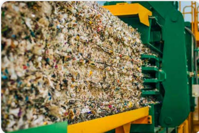
RDF is generally comprised of 30% - 40% plastic waste with the remainder a mix of timber, paper and textile waste that is uneconomic to recycle, but has high calorific value so that it burns. In Australia there are currently no standards or specifications for RDF, other than a minimum calorific value to ensure it can be burned by
