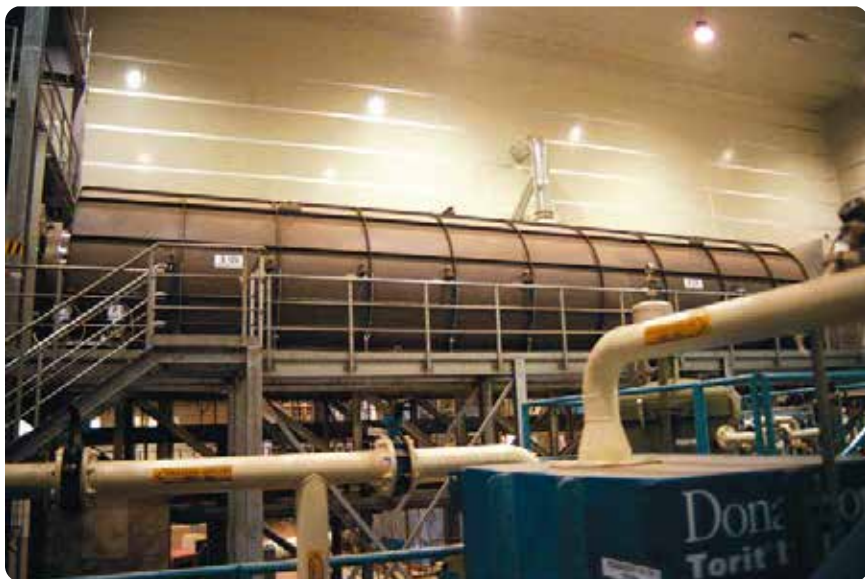
Figure 20. Indirect Thermal Desorption Unit (ITDU) Spolana Neratovice.
