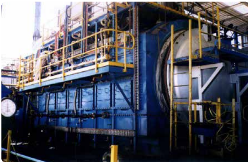
Figure 7. Thermal reduction batch processor (TRBP) of GPCR system. Source: D. Hallett
