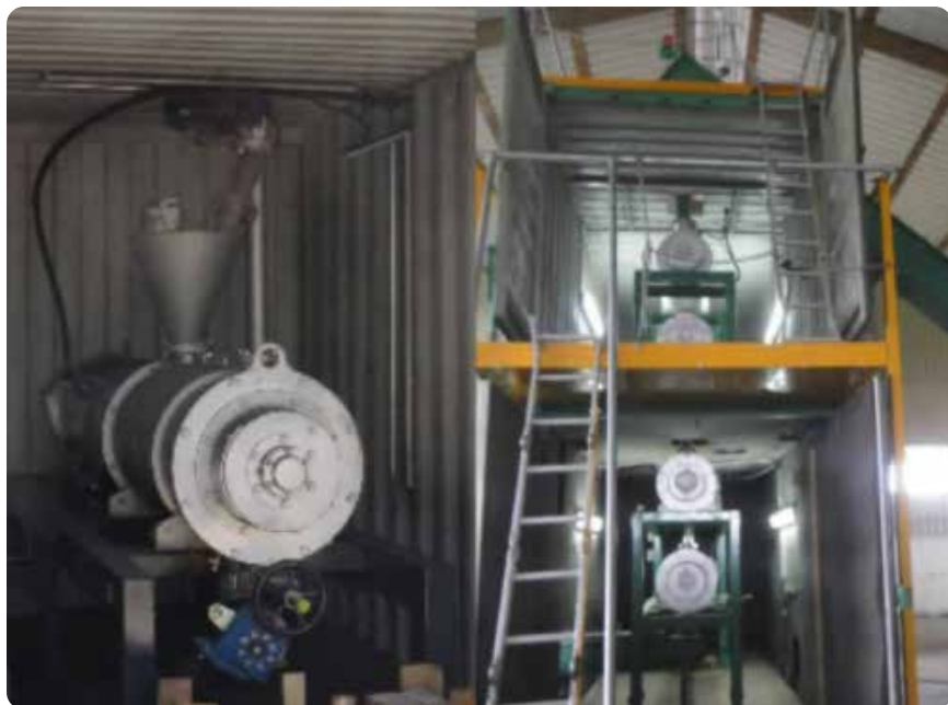
Figure 3. The compact and modular EDL ball mills are readily transportable to remote stockpiles. Source: EDL Europe
