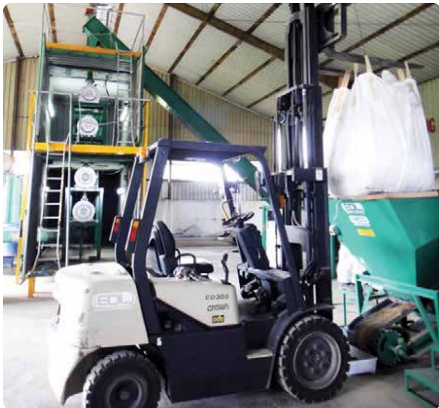
Figure 5. EDL ball mills treating high strength dioxin waste in Bien Hoa, Vietnam.
