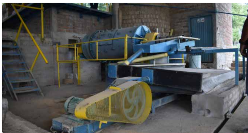
Figure 14. New mercury-free gold ore processing equipment purchased by the Cooperative at the Íquira mines. Source: Cooperativa Agrominera
