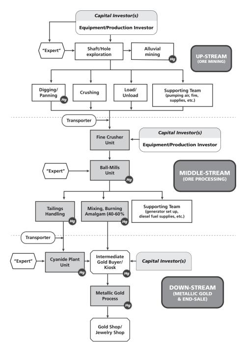
miners mine or dredge the ores from the bottom of the river and process the ore in sluice boxes with mercury above the river. The end-result is primarily a gold purity of approximately 20-60 percent..
