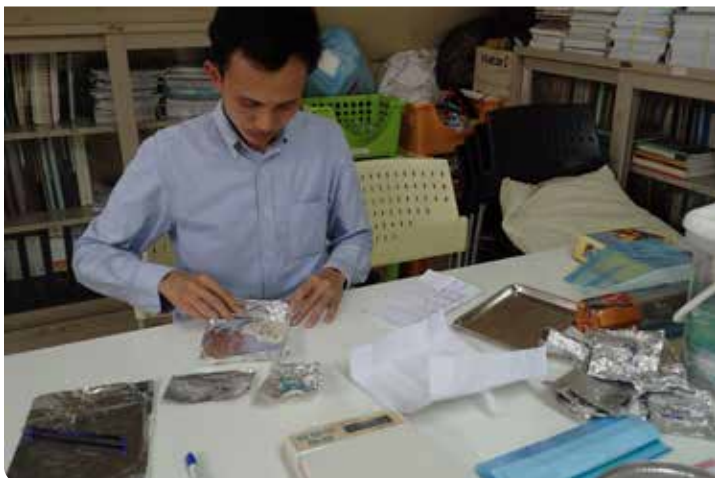
Sample Collection: Plastic waste at the high-tide line was sifted for plastic pellets. Roughly 100 pellets from each location were packaged, labeled, and sent for testing. Photos: Earth Thailand
