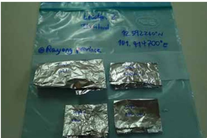
Sample Collection: Plastic waste at the high-tide line was sifted for plastic pellets. Roughly 100 pellets from each location were packaged, labeled, and sent for testing. Photos: Earth Thailand
