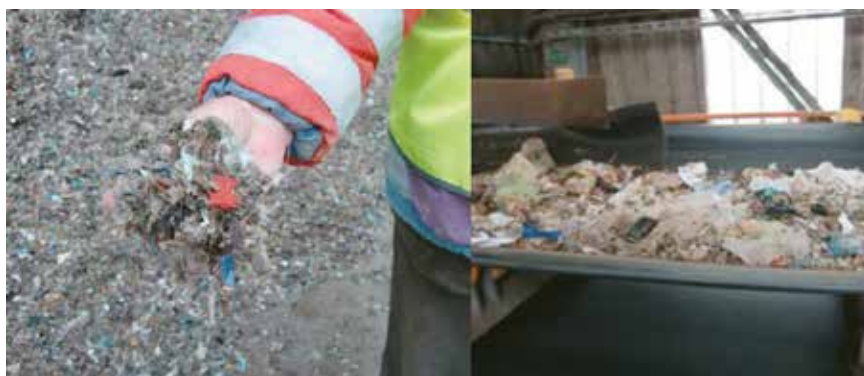
Figure 20. (a) Fine SRF for main burner; (b) Crude SRF for pre-calcination. Photo: Asosiasi Semen Indonesia, et al. (2017)
