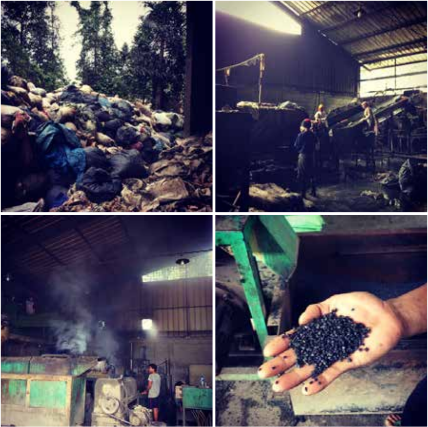
Figure 15. Plastic bags recycling. An SME outside Jakarta converts 30 tons of used plastic bags into 6 tons of PE pellets per day. Photos: Nexus3
