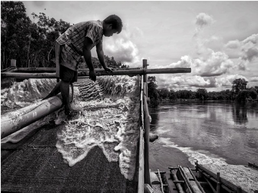
Fig. 5 Mercury poured into the carpet on of a sluice box in a river in Kalimantan. Photo credit: Larry C.Price/Pulitzer Centre on Crisis Reporting
