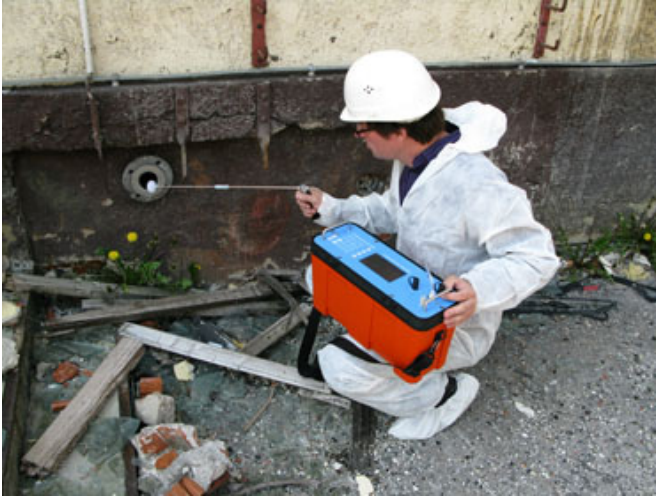
Picture 1. Example of a contaminated site investigator using a portable mercury vapour analyser. Source: www.mercury-instrumentsusa.com
