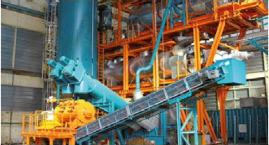
Picture 15. Indirectly heated vacuum distillation unit.
