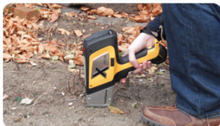
Picture 2. The Olympus Delta portable X-Ray Fluorescence Analyser with screen shot example of digital screen readout for metals in polymer. Source: www.innovx.com
