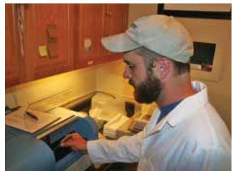
Samples were analyzed on BRI's Milestone DMA 890, using a U.S. EPA-approved method (SW-846 Method 7473).
