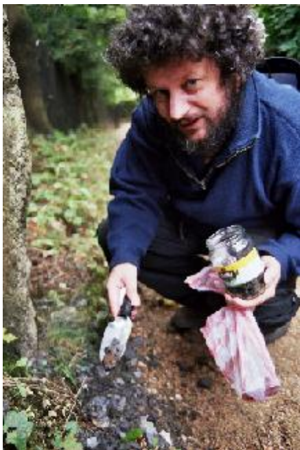
Photo No. 5: Fly ash and bottom ash mixture sampling at bicycle path in the Protected Landscape Area Jizerské hory.
