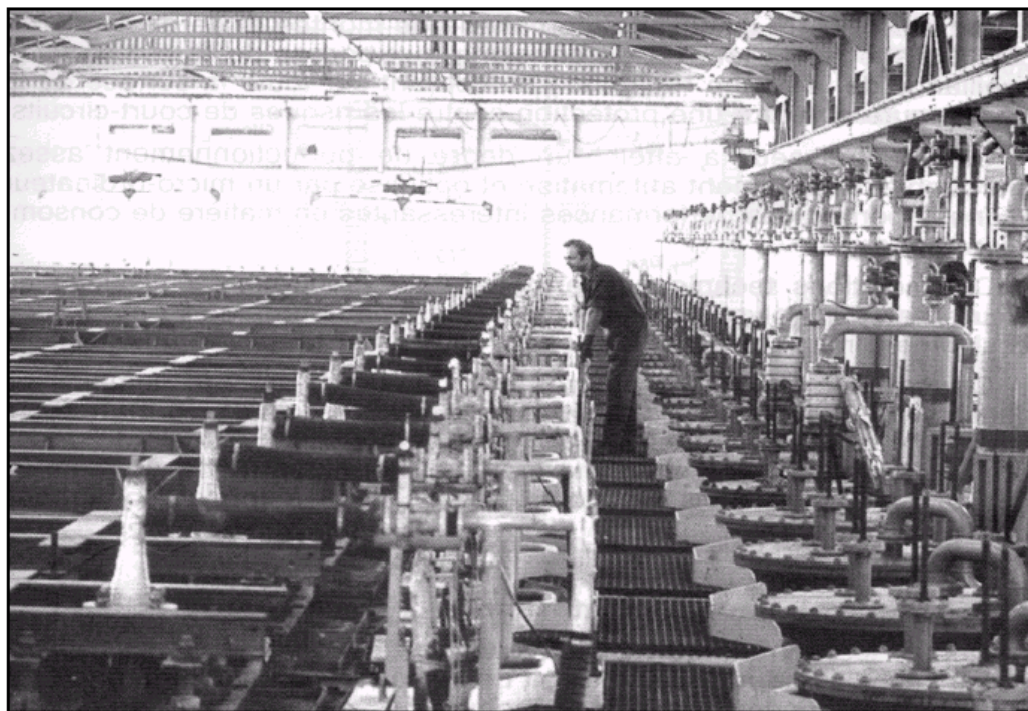
Figure 2.5: Mercury cells with vertical decomposer [Le Chlore, 1996]
