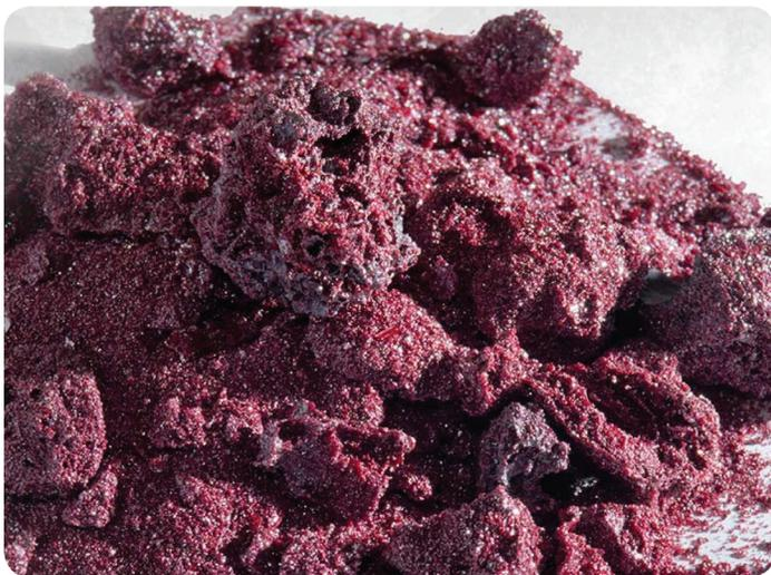
**Figura 3. Mercury 'retired' by sulphide stabilisation.**
